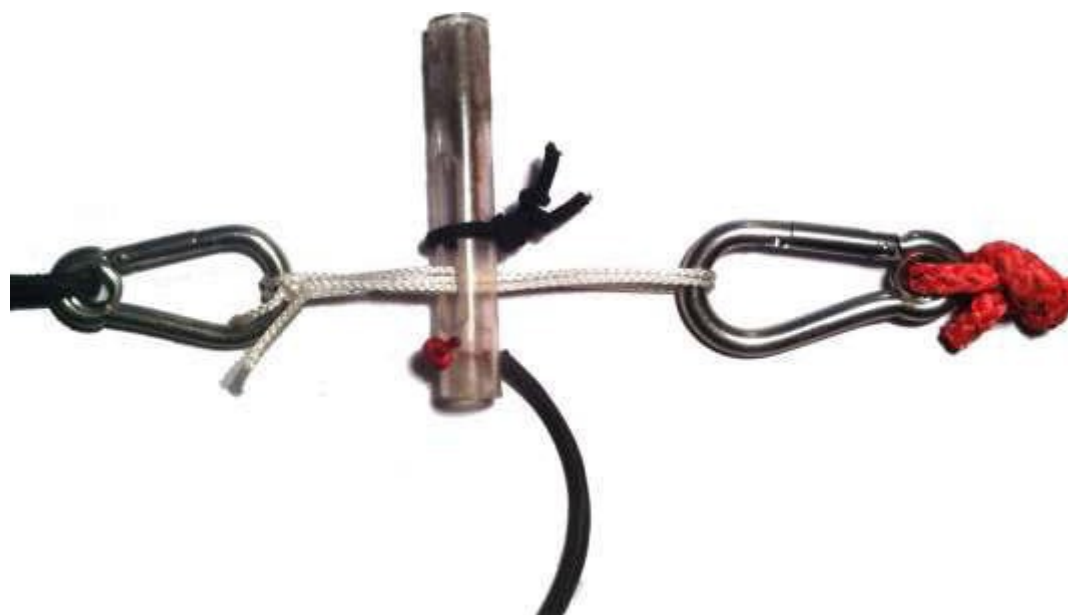
Figure 3 - Link Knife. In this photo, the o-ring has been replaced by a bungy cord.
