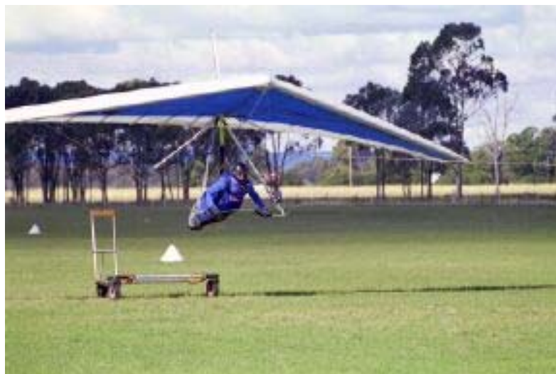
Pilot and glider launching aerotow out of the 'dolly'.
